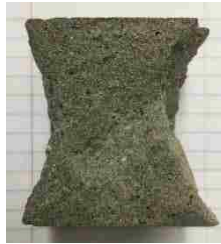
Figure B - 1. Failure Mode of Typical Mortar Cube (8/27/15) @ 28-day Failure
