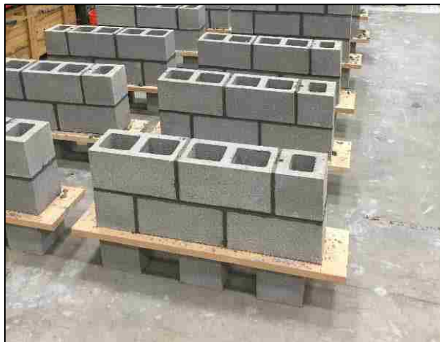
Figure 12. Wallettes Prior to Grouting
