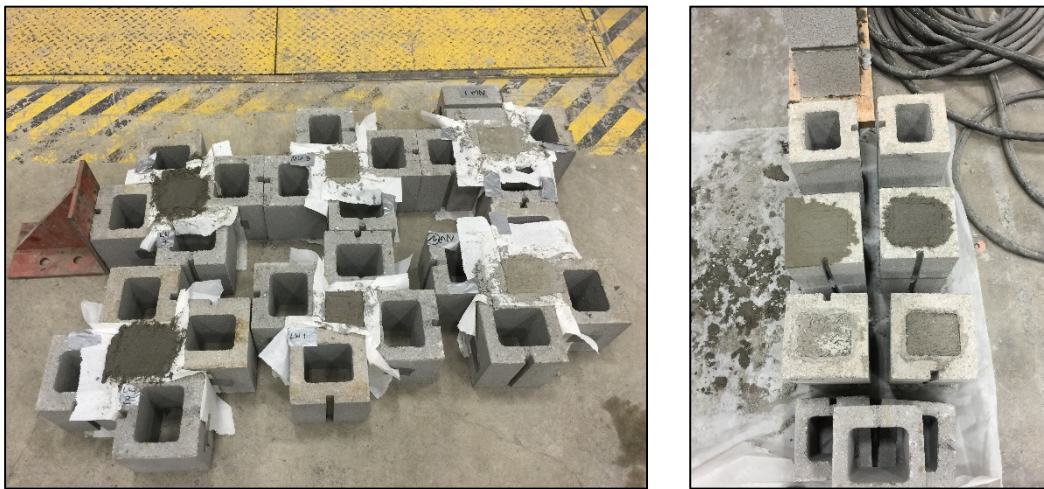
Figure 20. Grout and Masonry Prisms
